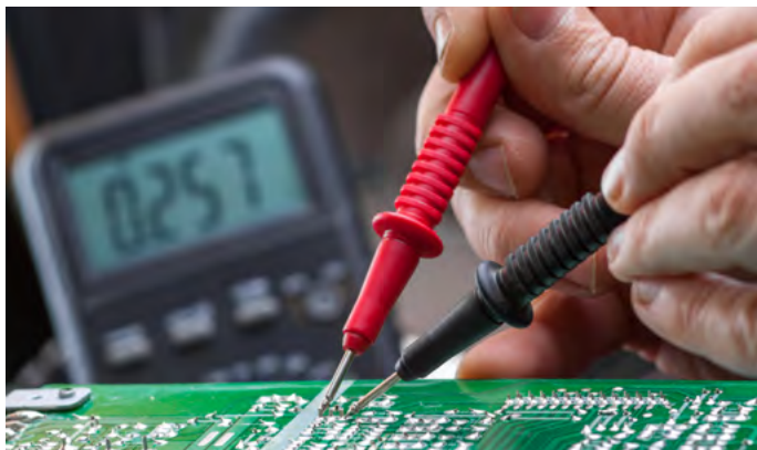
Manually Testing a Circuit Board
