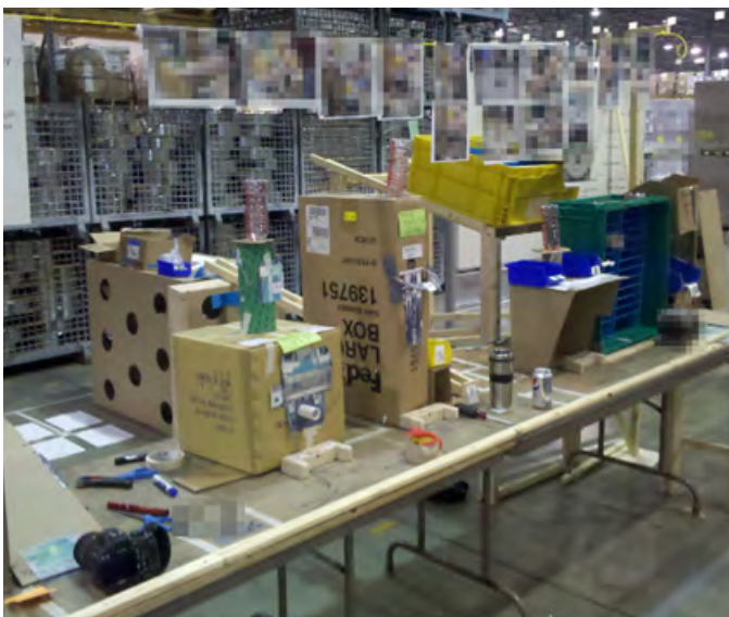
Example of a Mock of Production Cell layout using "Cardboard Machines"
